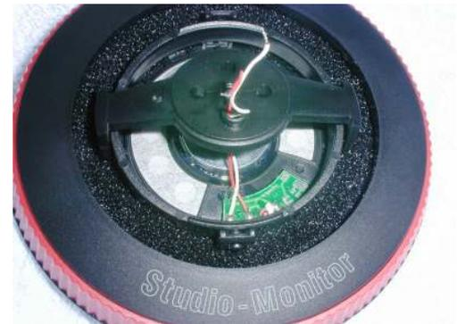
Pull the inner ring upwards and take it off including the paper damper-ring, now you can see the driver and soldering pads.
