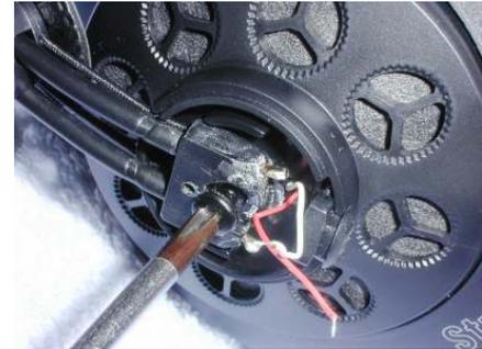
Make sure the wires go through the hole with the protruding rim and put the paper damper back and refit the ring. Mount the assembly back onto the headband and resolder the wires on the right spot. Refit the cap and nameplate.
