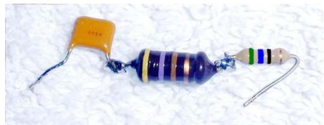
Solder the parallel filter (470 µH, 1µF and 39Ω) and the series filter (470 µH, 1µF and 56Ω)
