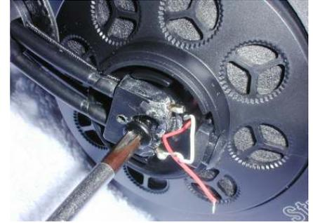
See and note where each wire was soldered on, desolder the wires and take out the screw.
