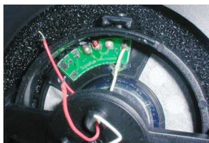
Carefully pry the red wire loose (glued with transparent glue) and desolder it.
